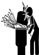
THIS FILTER OPERATES UNDER HIGH PRESSURE. WHEN ANY PART OF THE CIRCULATING SYSTEM (e.g., LOCK RING, PUMP, FILTER, VALVES, ETC.) IS SERVICED, AIR CAN ENTER THE SYSTEM AND BECOME PRESSURIZED. PRESSURIZED AIR CAN CAUSE THE LID TO BLOW OFF WHICH CAN RESULT IN SEVERE INJURY, DEATH, OR PROPERTY DAMAGE. TO AVOID THIS POTENTIAL HAZARD, FOLLOW THESE INSTRUCTIONS.
